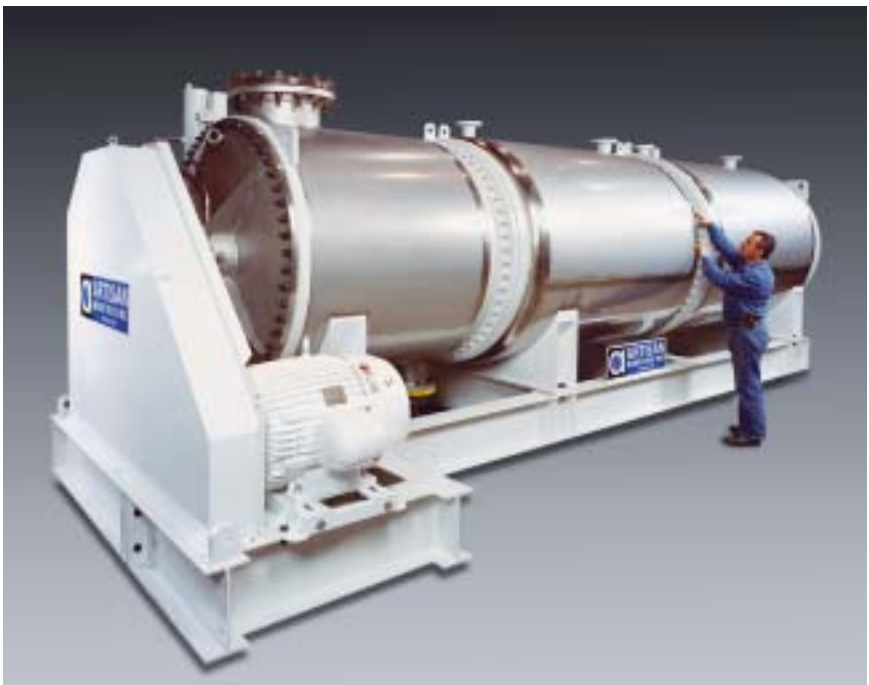
200 sq. ft. Rotothem® Horizontal Thin Film Evaporator
